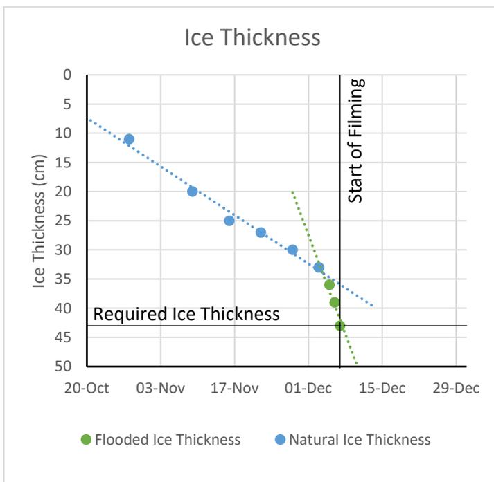
By the end of November it was evident that the recommended 43 cm of clear strong ice was not going to form naturally and that Mother Nature needed help. Tetra Tech assisted with the direction of clearing and flooding efforts for the project area measuring nearly 30 acres (600 x 200 m).
